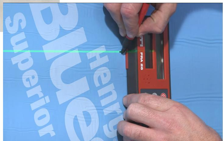
For this "example" elevation we have 3 different laser setups: vertical lasers (approximately 30' apart), horizontal laser (placed at a height that is comfortable to measure), and a plane laser (set out 3" – 6" off the face of the substrate or bar). The plane laser will be used to measure to face of bar or substrate, face of window and doors.
