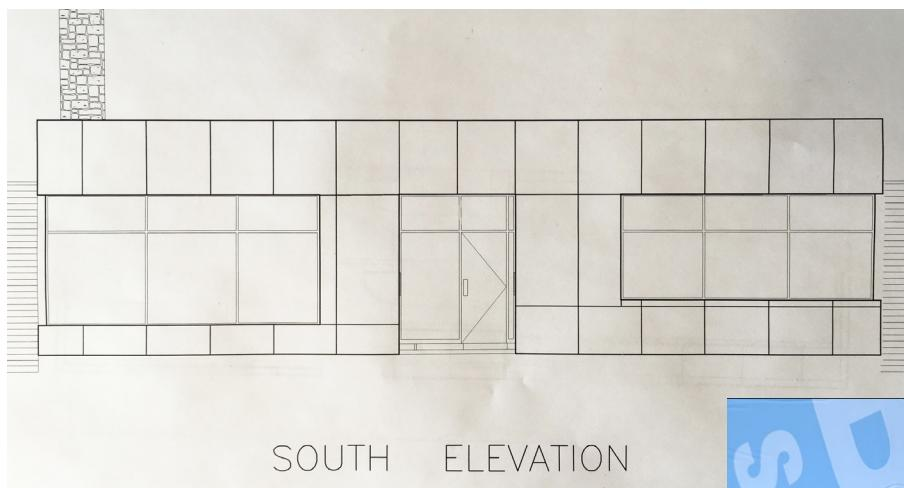
A blank set of architectural elevation drawings are used similar to the example below. These drawings show top and bottom of wall, window and door openings. These drawings are clear of all dimensions and text which allows for the site dimensions to be clear and visible.
