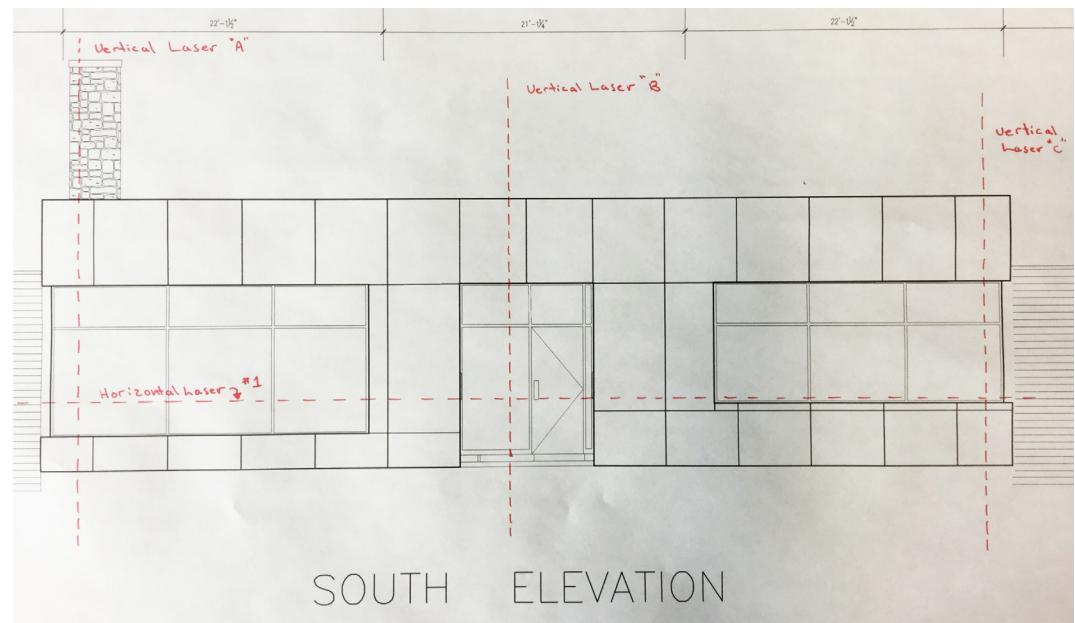
The "example" elevation is constructed of plywood sheathing; the windows and doors are commercial window wall. This is the most commonly used glazing system and depending on the stage of construction you may be measuring to different components of the curtainwall. Many acronyms are used throughout the measuring process to keep the drawing free of clutter. See example below of a mullion cap section and common parts that are labelled.
