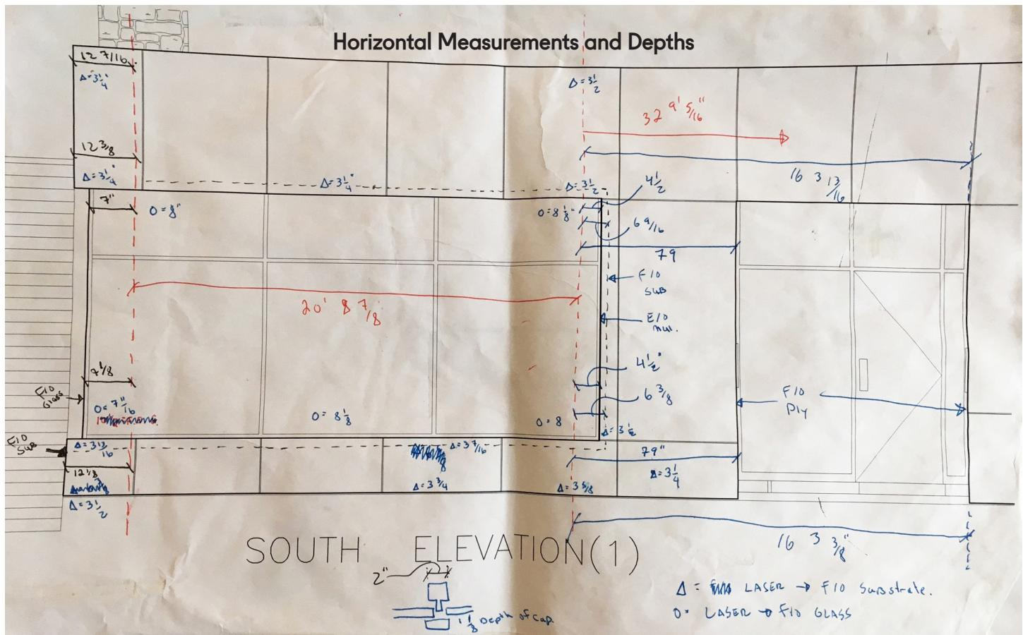
\*note the triangle and circle symbols at the bottom of the page that represent depths from the plane laser to face of substrate and glass\*
