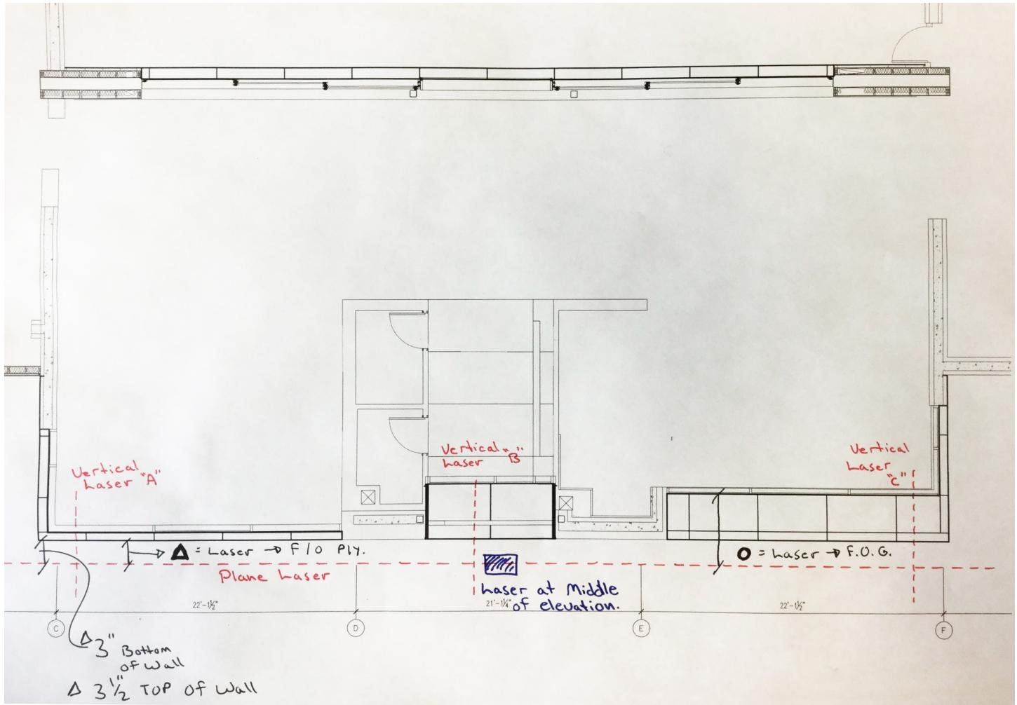
All laser lines will be labelled on your site dimension drawing and submitted for design. Upon the delivery of fabricated panels you will receive a copy of installation drawings. These drawings will have your laser lines marked on it and are to be used as a reference to begin a successful installation.
