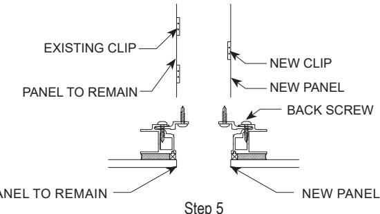
Attach the MC4 connectors of the new panel to where the old panels MC4 connectors were disconnected from. Place the new panel into place and fasten the half clips to the subframing.
