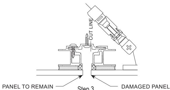
Remove the panel that needs replacement. During this step, unbuckle the MC4 connectors on the backside of the panels from panel/ optimizers.
