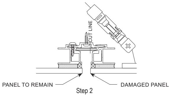
Locate wiring between panels. Note location for avoidance during step 4. Cut clip between the fastener and the panel to be removed. Make sure not to cut on the wrong side of the screw.
