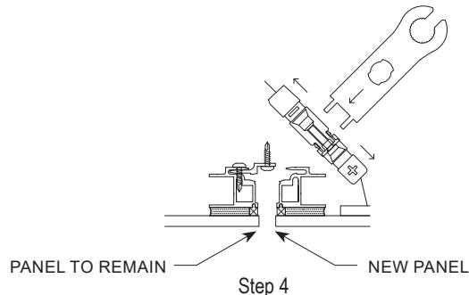
Back screw the half clips to the perimeter extrusion of the new panel. Make sure they are not at the same location as existing clips on the wall.
