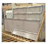
Skids and crates are custom built to ship panels to every project. Panels are numbered, packed and shipped in sequence based on the predetermined plan for installation.
